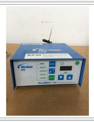
These controllers insure the main control of the deposit size.
